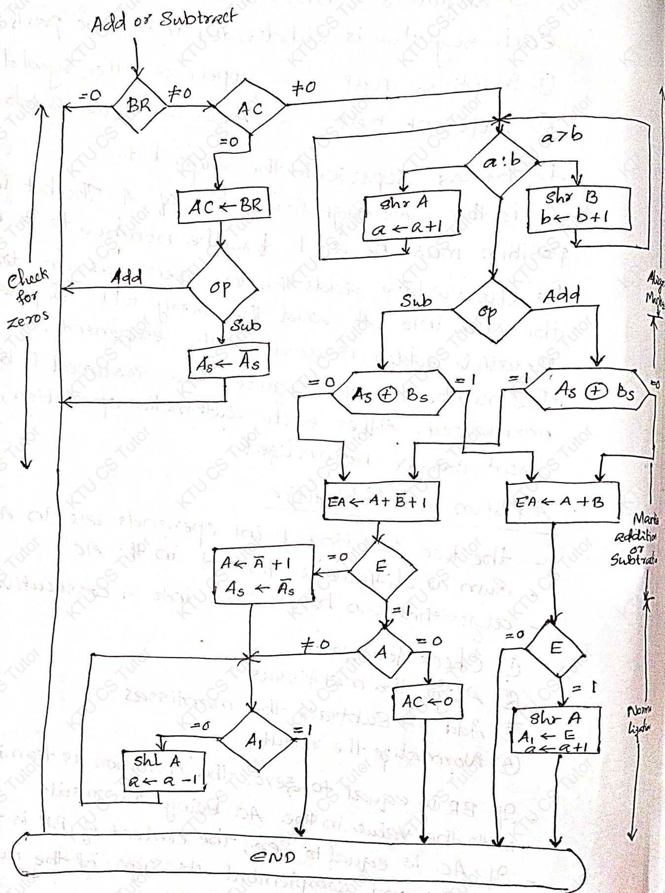
If the two exponents are not equal, the mantissa having smaller exponent is shifted to the right and its exponent incremented. This process is repeated until the two exponents are equal.
